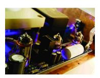
The CD-77 has as standard analog RCA and balanced XLR outputs, to ensure compatibility with any balanced equipment. At the same time, to maximize the sound quality, the designers kept to a single-ended electronic circuit throughout.
