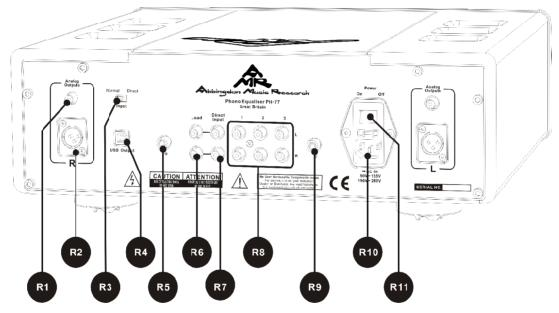
R1. RCA outputs: for the connection of RCA interconnection cables.
