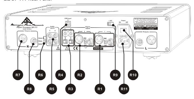
Always power OFF before changing an input selection R1 & R2. Input 1/2: "HD-Valve Digital Input" Digital SPDIF BNC/XLR (switchable): able to accept standard XLR SPDIF signal of 5Vpp OR BNC standard SPDIF signal of 500mVpp.
