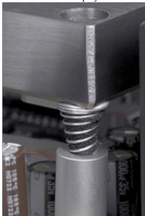
The heavy Transport Block floats on four of these springs
