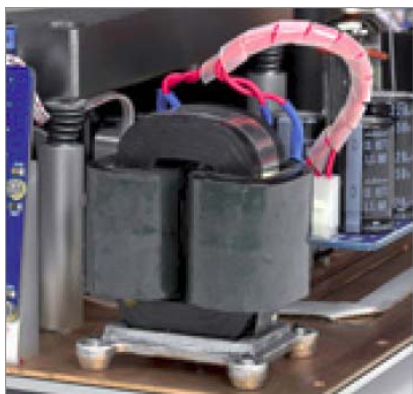
Filter Chokes for the elaborate power supply for the Valve output stage
