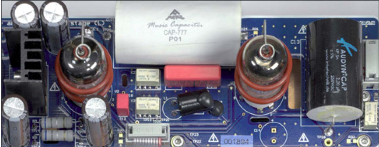
As standard the player comes with NOS Valves, sitting below holding clamps and fitted with anti-microphonic rubber rings
