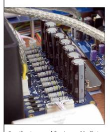
Rectification, amplification and buffering: no lack of cutting-edge components in the AMR, as the SMD rectifying diodes at the front, evidence.
