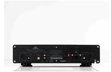
In the CD-777, the manufacturer has fitted traditional RCA-connectors and an XLR output as well, all the while, maintaining a single-ended circuit throughout.
